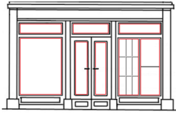
Sign Measurements-The areas outlined in red indicates a single window frame section
