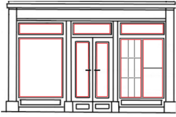
Sign Measurements— The areas outlined in red indicates a single window frame section.
